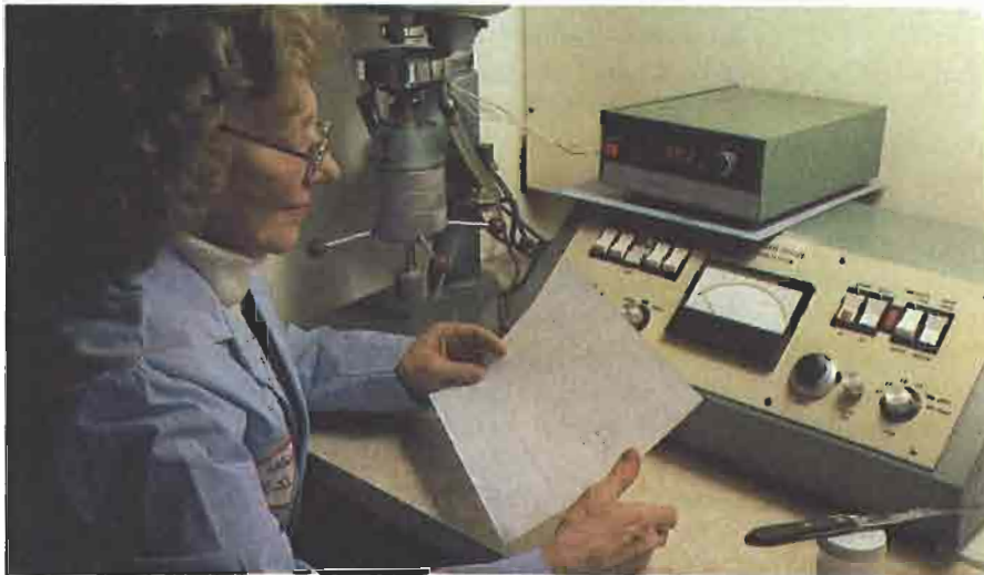
Fig. 3 Shirley Ferranti viscometer used to determine the viscosity of liquid bright gold by automatically plotting data from which rheological properties can be calculated
