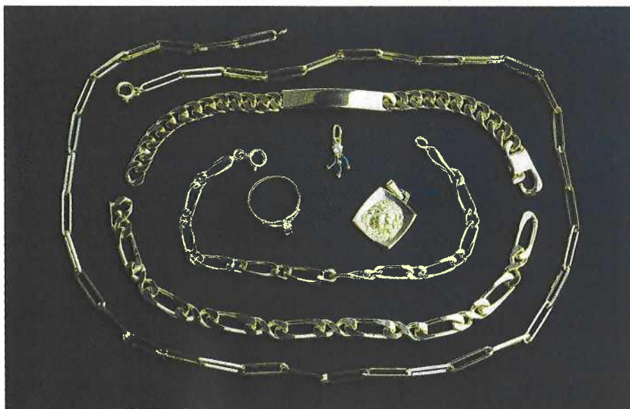
Fig. 4 Gold-plated vermeil jewellery (2 µm gold-cobalt plus 15 µm gold-copper-cadmium on sterling silver).
