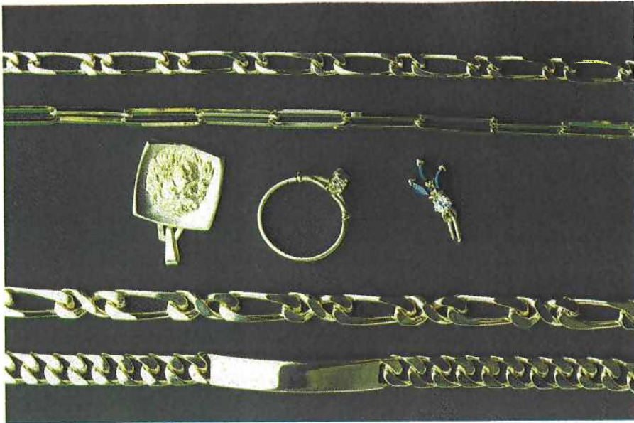
Fig. 1 Gold-copper-cadmium plated jewellery (20 \mu\text{m} thick).
