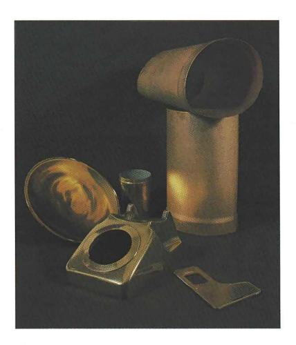
This photograph illustrates the decorative potentialities of aerosolsprayed electroless gold coatings and shows the fully bright, as-deposited surfaces that may be obtained by the process developed by Fulmer Research Laboratories on articles of various materials, topographics and sizes
