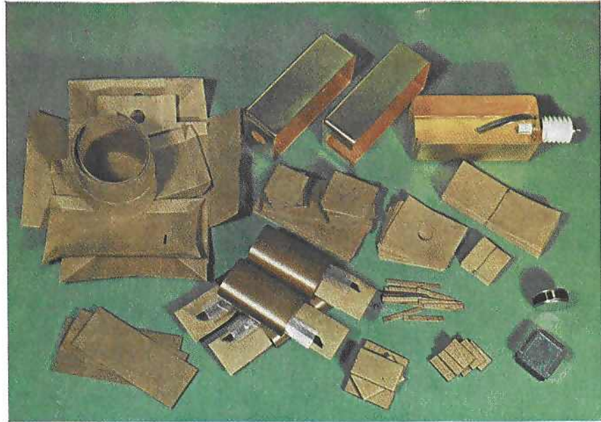
Fig. 3 The parts of a high voltage paper capacitor used in repeaters manufactured by Standard Telephones & Cables. They include four elements comprising moisture-free paper with aluminium foil electrodes (below centre), paper liners and packing pieces, a small bellows (below right), and the gold-plated copper cans (above right)
