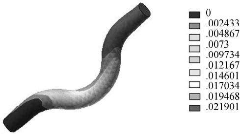
图 2 弹簧管不同点的位移量(@20 MPa) Fig. 2 The deformation of the spring tube(@20 MPa)
