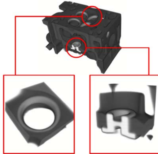
Fig. 9. CT data of a car engine-head which contains aluminum parts (gray areas) and iron parts (white areas). Specially, we extracted two multi-material areas from the data for experiments.
