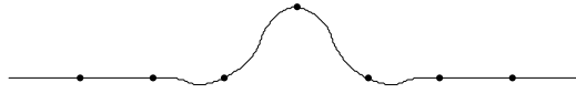
Fig.3. Result of the 3-point ternary scheme after four subdivision steps with w_j^k \equiv \frac{1}{4} .
