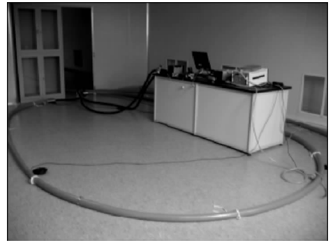
Fig. 2 Installation diagram rabbit system
