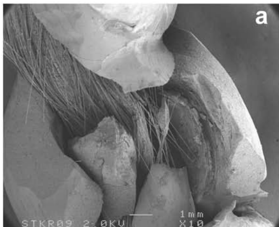
Fig. 2 Representative SEM pictures after fracture strength test: (a) everStick-Clearfil Photo Posterior FPD. Note the delamination of the veneering resin into mainly two pieces; (b) Ribbond-Clearfil Photo Posterior FPD. Note the catastrophic delamination of the veneering resin (original magnification \times 10 ).
