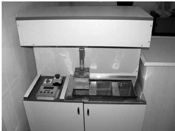
Fig. 1 Electronic thermal cycling machine used in this study.
