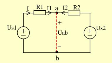
$Uab=Us_1-R_1I=1-1 \times 1=0V$ ;  $I_1=1A$ ;  $I_2=-1A$ ; Iab=0A
