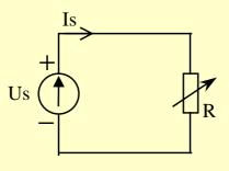
maintains its current, the voltage is determined by the load
