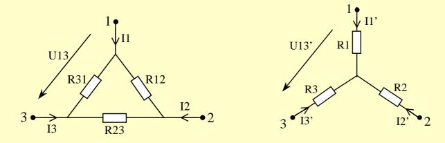
$$R_{1} = \frac{R_{31}R_{12}}{R_{12} + R_{23} + R_{31}} \qquad R_{2} = \frac{R_{12}R_{23}}{R_{12} + R_{23} + R_{31}} \qquad R_{3} = \frac{R_{31}R_{23}}{R_{12} + R_{23} + R_{31}}$$
