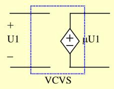
VCVS: A voltage-controlled voltage source
