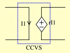
CCVS: A current-controlled voltage source
