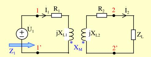
$$Z' = \frac{(\omega M)^2}{R_{22}^2 + X_{22}^2} (R_{22} - jX_{22}) = (218 - j1904) \Omega$$
