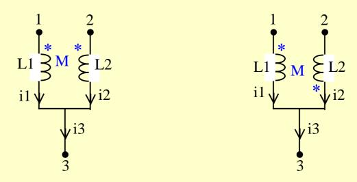
$$\begin{split} u_{13} &= L_1 \frac{di_1}{dt} \pm M \frac{di_2}{dt} \,, \quad u_{23} = L_2 \frac{di_2}{dt} \pm M \frac{di_1}{dt} \\ \vdots \\ U_{13} &= j\omega L_1 I_1 \pm j\omega M I_2 \,, \quad U_{23} = j\omega L_2 I_2 \pm j\omega M I_1 \end{split}$$
