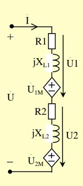
$$\dot{U}_1 = \dot{I}(R_1 + j\omega L_1 \pm j\omega M)$$
