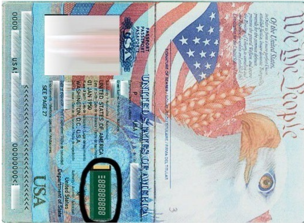
Fig. 2. Sample ePassport with a Display Unit
