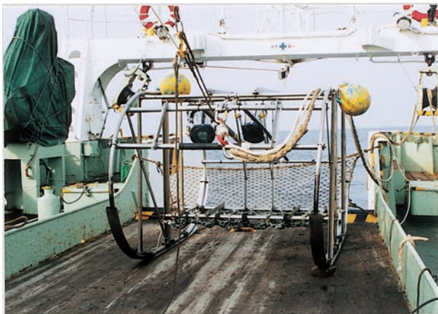
Fig. 1. The deep-sea video monitoring system on a towed sledge on the R/V Kaiyo-maru No. 3
