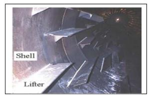
Figure 3. The inside view of a normal rotary dryer.
