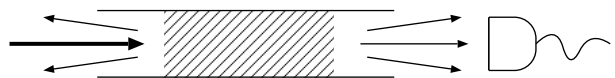
FIG. 1. Monochromatic radiation (thick arrow) is incident on a disordered absorbing medium (shaded), embedded in a waveguide. The transmitted radiation is measured by a photodetector.
