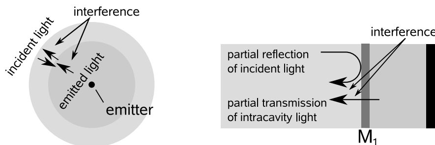
FIG. 2: Comparison of the interferences of light beams in the case of complete illumination of the systems.
