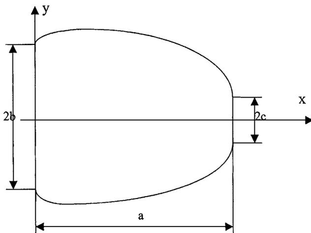
FIG. 3. A symmetric, parabolic, trapezoidal plate.
