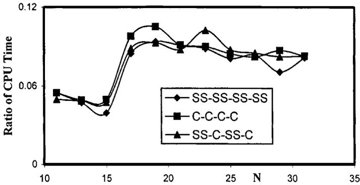
FIG. 7. Ratio of CPU time (present/reference [6]) versus  $N (=M)$  for vibration analysis of eccentric sectorial plates.
