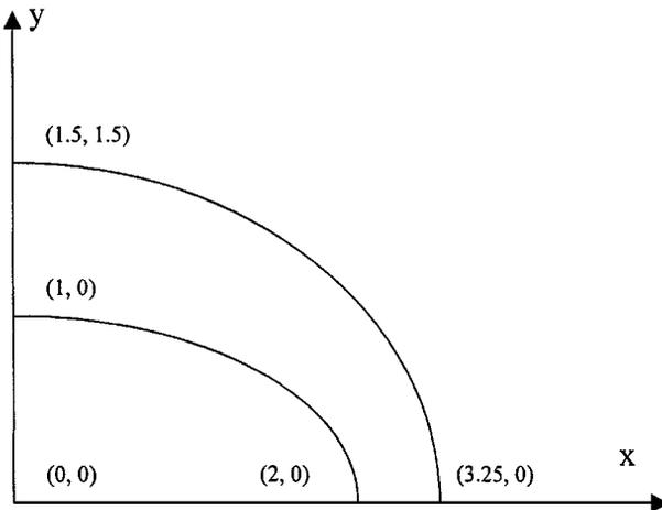
FIG. 5. A quarter section of an elliptical plate.
