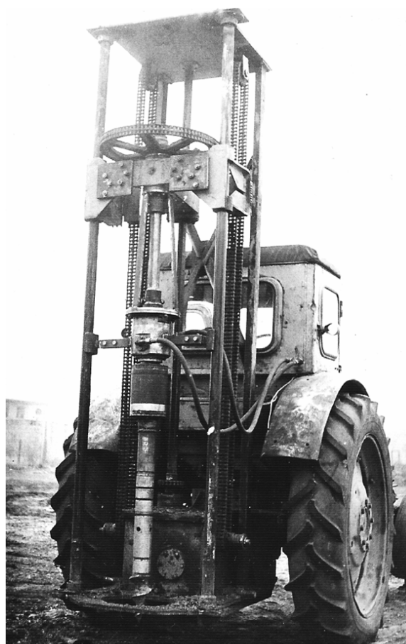
Fig. 1. Standard working equipment of gasodynamic soil loosening machine
