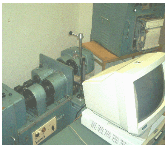
Fig. 2. Friction-wearing machine SMC-2
