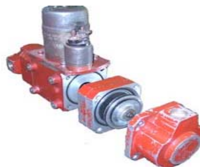
Fig 2. Piston suction pump driven by electromotor
