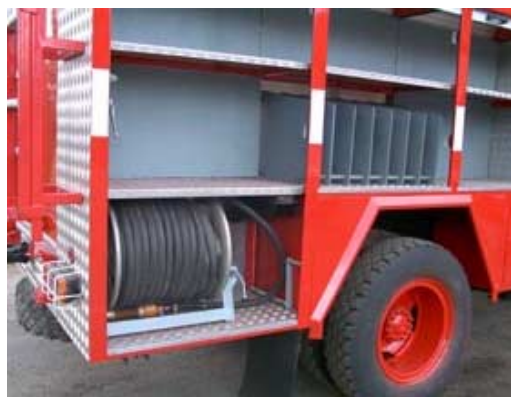
Fig 4. Mounting of the fast response hose on the fire vehicle with the new body construction
