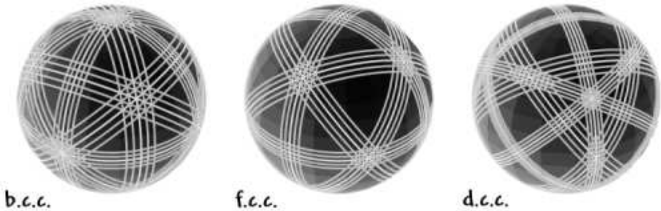
FIG. 6: Visibility maps for the two largest fringes visible from body-centered, face-centered, and diamond face-centered lattices. Sphere diameter (relative to band width and fringe spacing) is proportional to specimen thickness, here chosen to be about 5 times the cubic cell side a . Note the dominance of crossed (110) fringes at the three-fold (111) zone in the body-centered case, the dominant crossed (111) fringes at the two-fold (110) zone in the face-centered cases, and the wider disparity between largest and next-to-largest spacings when the diamond glide is added to the lattice.
