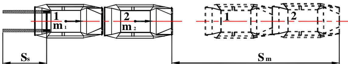
Fig 2. Scheme of direct collision when both cars are braked
