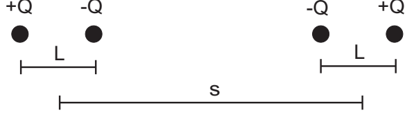
Figure 8: Superconducting pendula under the influence of tidal forces that produce charge separation. The Physical dimension of the pendulum along the axis of the charge separation is given by L , and the center-to-center distance between the pendula is given by s .
