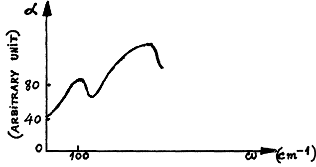
FIGURE 1 Optical absorption coefficient of a -Ge; this plot is experimental (after Ref. [6]).
