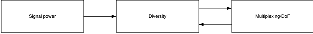
Fig. 1. An indirect approach to achieve interference alignment via varying signal power to provide more diversity.
