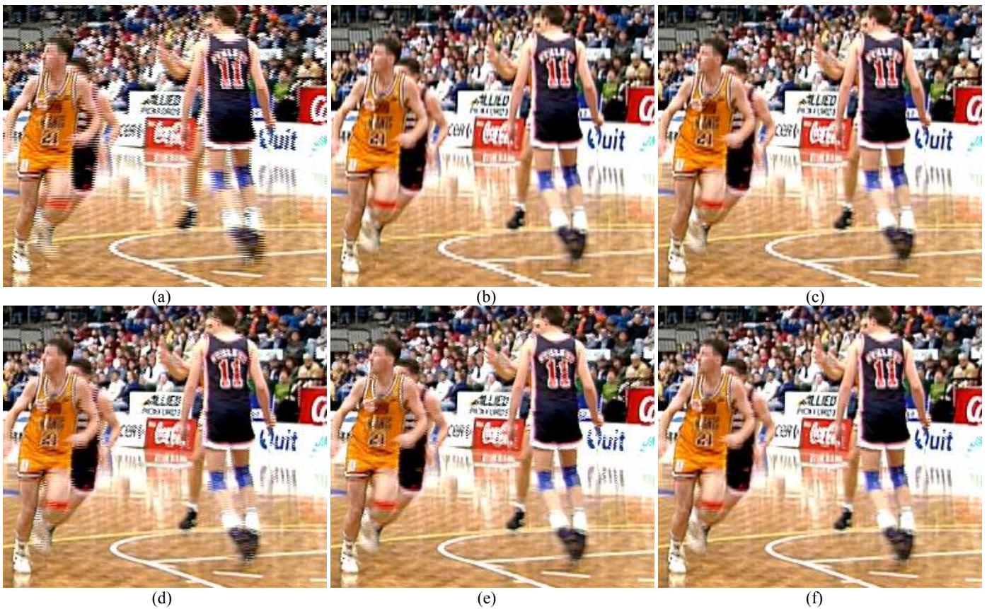
Fig. 9. Subjective performance on the Basketball sequence with SD resolution. (a) “Weave” [23], (b) LA, (c) AR, (d) sub-pixel EMF, (e) LSTF + median filtering, (f) proposed adaptive deinterlacing technique selectively using two kinds of motion estimation.
