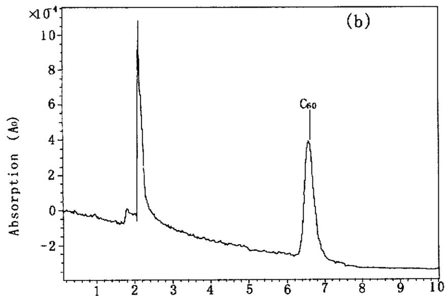
图1 样品03# (a)抽提物与参考物质纯C<sub>60</sub>(b)的HPLC对照分析结果Fig.1 HPLC chromatograms derived from 03# (a) and C<sub>60</sub> reference material (b)
