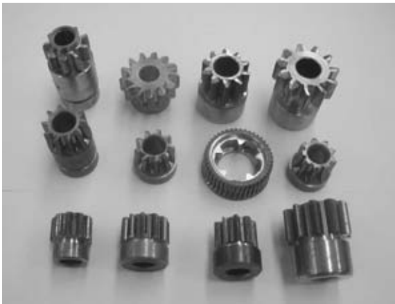
Fig. 1. Cold formed steel forgings from ISKRA Avtoelektrika production program. Testing forging – pinion no. 16.920.633 (below, the second from the left)
