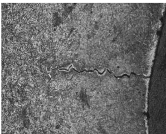
Fig. 5. Tooth – sample D. Surface layer, crack through the surface layer; magn. 500x; OM
