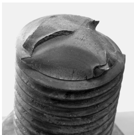
Fig. 4. Destroyed M42 bolt from flange joint
