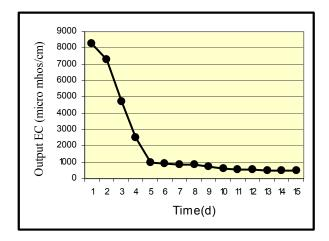
**Fig. 2:** EC variations in effluent water (in constant input EC: 500 μmohs/cm)
