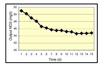
**Fig. 4:** Nitrate variations in effluent water (in input nitrate: 45.5 mg/l)
