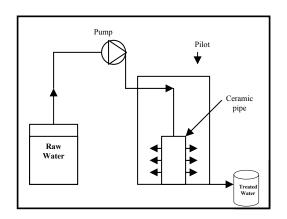
Fig. 1: Schematic design of the pilot
