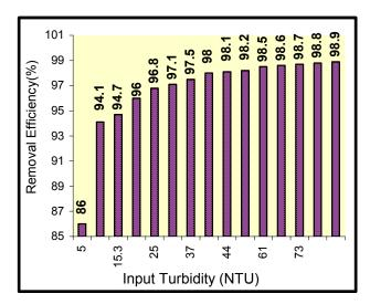
Fig. 5: Efficiency of system in turbidity removal
