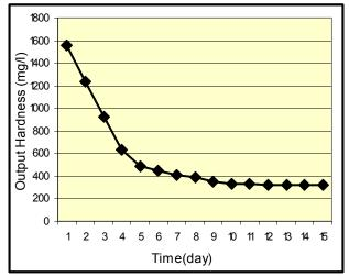
Fig. 6: Hardness variations in effluent water (in constant input hardness: 300 mg/l)
