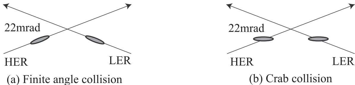
Figure 4. Collision schemes at KEKB: (a) finite angle collisions and (b) crab crossing.
