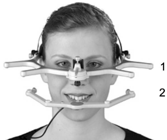
Figure 1. The JMA-System mounted on the head of a patient. 1: Lower frame with three built-in ultrasonic transmitters, fixed with a functional occlusion metal clutch to the lower anterior teeth. 2: Upper frame with four built-in receiving sensors (reproduced with the kind permission of Zebris Medical GmbH, Isny, Germany).
