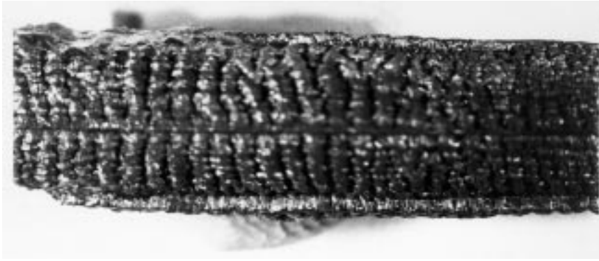
Figure 6. A well-defined hot zone forms at positive electrode and travelled along the rod and disappeared on reaching the negative electrode leaving a corrugated surface on the rod.
