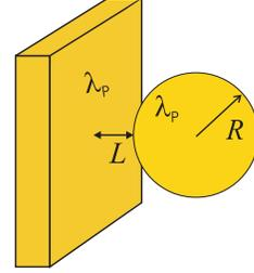
FIG. 1: The geometry of a sphere of radius  $R$  and a flat plate at a distance  $L$  (center-to-plate distance  $\mathcal{L} \equiv L + R$ ); both mirrors are covered with a metal characterized by a plasma wavelength  $\lambda_p$ .
