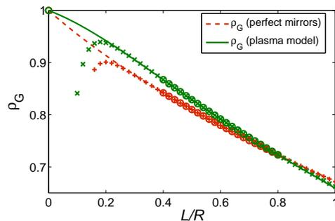
FIG. 3: Quartic polynomial fit of the function  $\rho_G(L/R)$ , for a nanosphere of radius  $R = 100\text{nm}$ ; the solid green line corresponds to gold-covered plates and the dashed red line to perfect reflectors. The crosses represent numerically evaluated points and the circles indicate those points which are used for the fit [Colors online].
