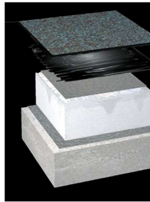
Fig. 3. – Performance system for renovation based on bitumen.
