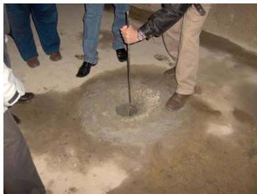
Fig. 5. – Borehole through floating slabs of the Civil Defense Shelter.
