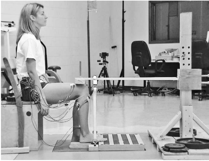
Figure 1. Triceps surae maximal voluntary isometric contraction assessment. The wooden plank was fixed rigidly to a force plate. The hip, knee, and ankle joints were oriented at 90° of flexion, and the metatarsal heads were placed on the top surface of the wooden plank such that plantar-flexion force was captured in the vertical ground reaction force. The position of the triceps surae loading device was held constant using a winch so that isometric triceps surae contraction could be produced. Reprinted from Clinical Biomechanics (Bristol, Avon) with permission from Elsevier. 22
