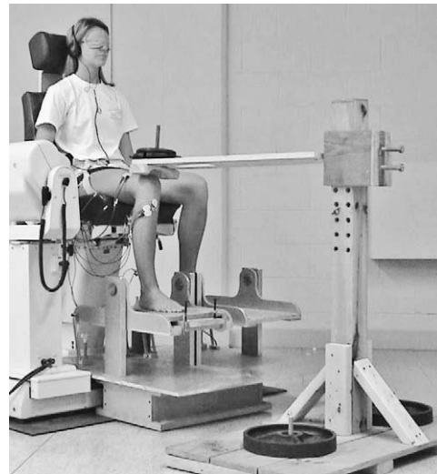
Figure 4. Spinal stretch reflex assessment. The applied load and lower extremity kinematics were identical between musculotendinous and spinal stretch reflex assessments. Reprinted from the Journal of Electromyography and Kinesiology with permission from Elsevier. 22
