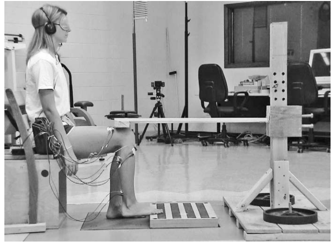
Figure 2. Participant positioning for stiffness assessments and determination of applied load. Rigid fixation of the wooden plank to the force plate allowed oscillatory motion of the system to be characterized in the vertical ground reaction force (GRFv) during stiffness assessments. The applied load was determined by adding mass until the GRFv equaled 30\% \pm 5\% GRFv max obtained during triceps surae maximal voluntary isometric contraction assessments. The vertical arrow indicates the application point for the downward manual perturbation force used to initiate oscillatory motion during stiffness assessments.
