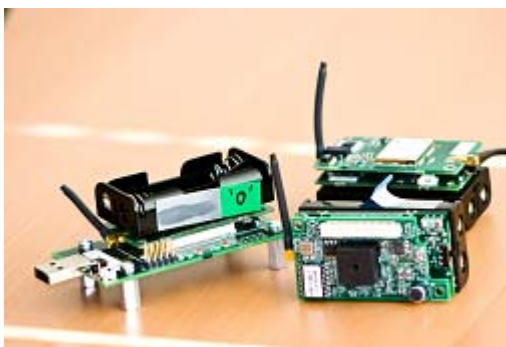
Figure 3: Wireless Multi-Sensor Nodes are Starting to Integrate GPS Technology which Enables Geolocation of the Nodes and their Data.
