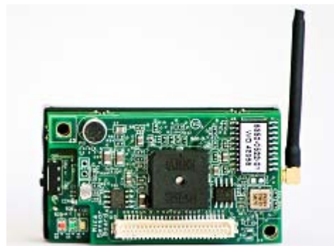
Figure 3: Wireless Multi-Sensor Nodes are Starting to Integrate GPS Technology which Enables Geolocation of the Nodes and their Data.
