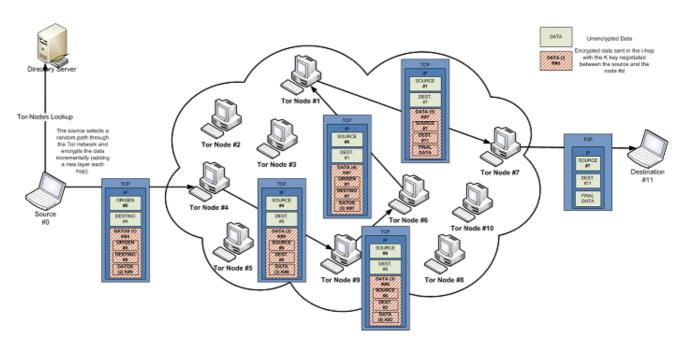
Figure 2: Tor Network. The source establishes an anonymous communication with the destination through a set of randomly chosen nodes, and incrementally encrypts the message by adding a layer each hop.
