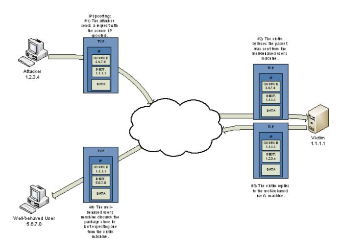
Figure 1: IP Spoofing. The figure shows how the attacker spoofs the source field of the IP packet so it will not be stated as a source of communication.
