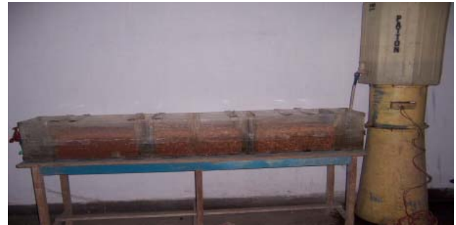
Figure 1. Model of horizontal roughing filter used in the experiment.
