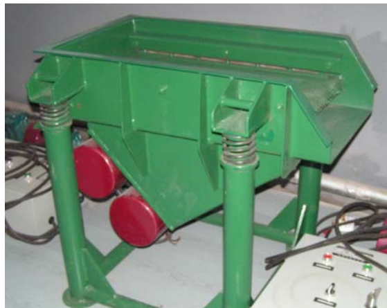
(a) Photo of a vibratory screener in laboratory, Type ZZS40-70
