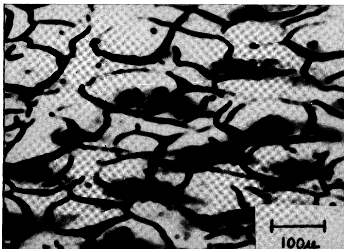
FIGURE 4 The cracks observed on the MA-600 carbon black/epoxy resin resistor.
