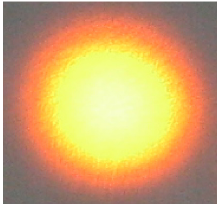
Fig. 6. The far field beam profile of the 589 nm yellow laser.
