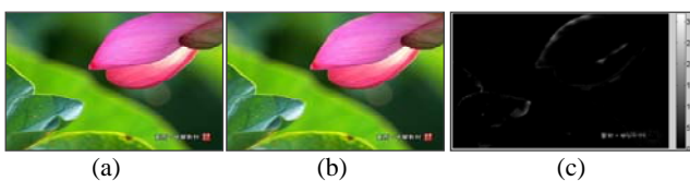
Figure 11. The improved 180Hz algorithm avoids the redundant lights propagating through the first field-image and maintains image fidelity. (a) The test image, Lotus , (b) simulated images after the improved 180Hz Stencil-FSC processing, and (c) CIEDE2000 error images.
