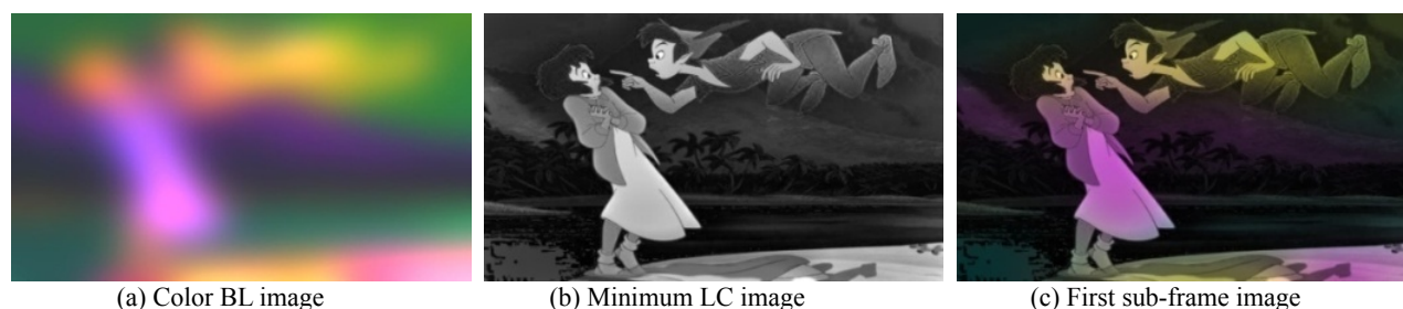
Figure 3 - Simulation results of the first sub-frame image. (a) A color backlight image, (b) a minimum LC image, and (c) the first sub-frame image.
