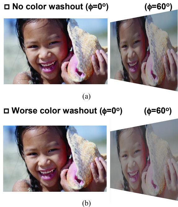
Figure 1. The photograph of (a) conventional MVA and (b) AMVA viewed from normal, right, and left sides.
