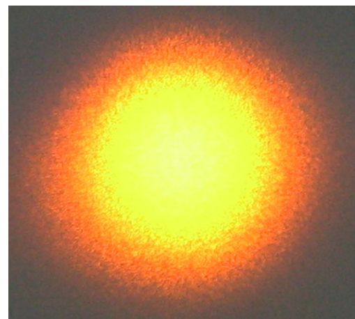
Fig. 6. Far field beam profile of the 588 nm yellow laser.
