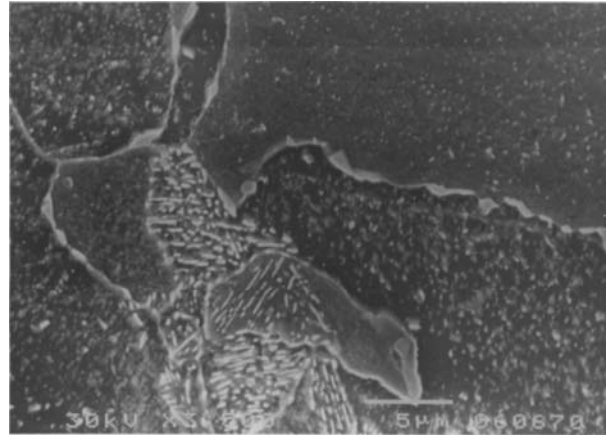
Fig. 4. Structure of the investigated cast steel after normalization and high tempering, nital etched
