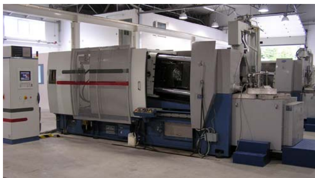
Fig. 1. Die casting machine for Mg alloys. See from the right: furnace, injection system, locking system with die, control desk.
