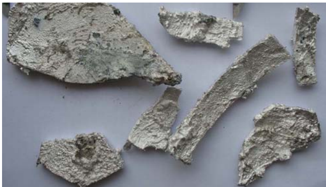
Fig. 3. Plates removed from the crucible bottom during casting of magnesium-based AZ91 alloy.
