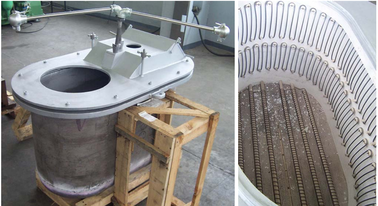
Fig. 2. Crucible for melting of magnesium alloys - left; furnace interior– right.
