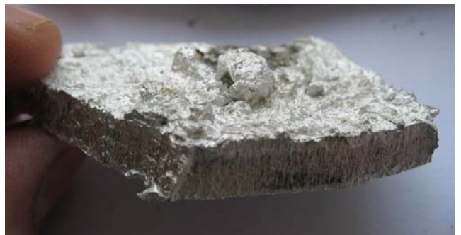
Fig. 4. A fractured specimen of the examined plate.
